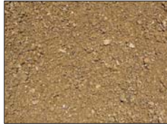
DECOMPOSED GRANITE SURFACE
