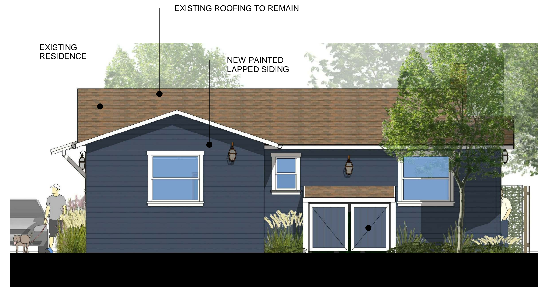
2 EAST ELEVATION - (E) HOUSE 1/4" = 1'-0"
