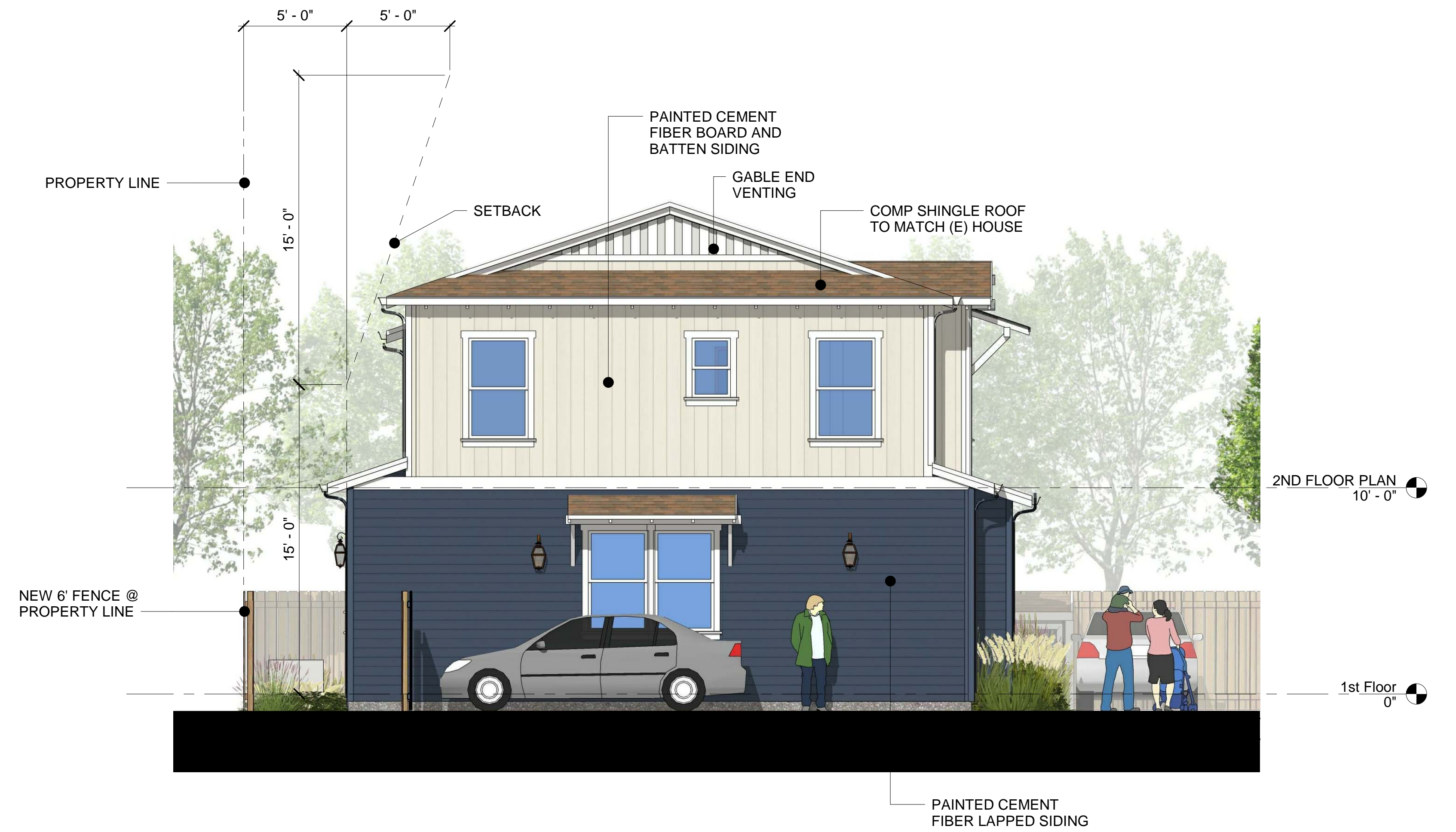
4 WEST ELEVATION - UNIT 1 1/4" = 1'-0"
