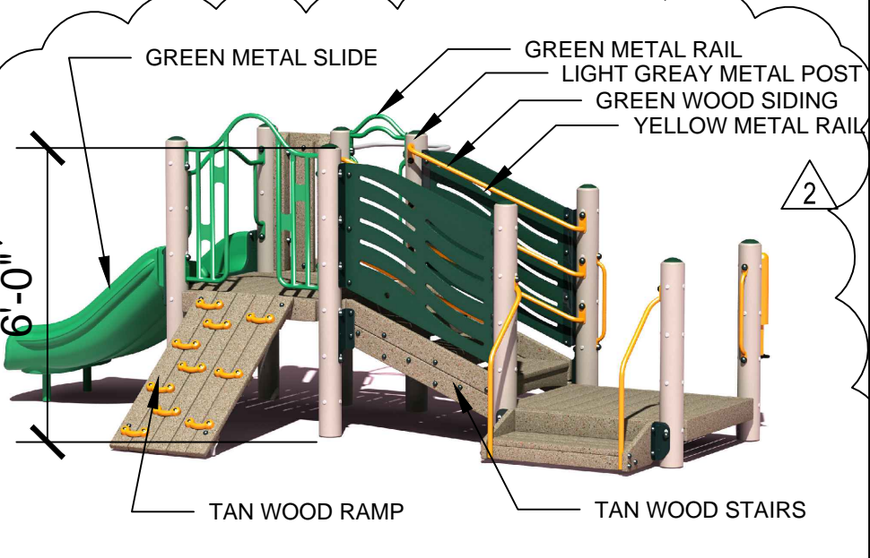
A LOW PLAY STRUCTURE SEE 9/C1.3 & 11/C1.3 FOR DETAILS
