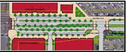
allows easier entry and exit from the on street parking. The bike lane is located away from the angle parking on the "through" section of Owens Drive. This separation of the bike lane from the on street angle parking eliminates a safety hazard that exists between vehicles backing out of angle parking and cyclists riding adjacent to the parking lane.
