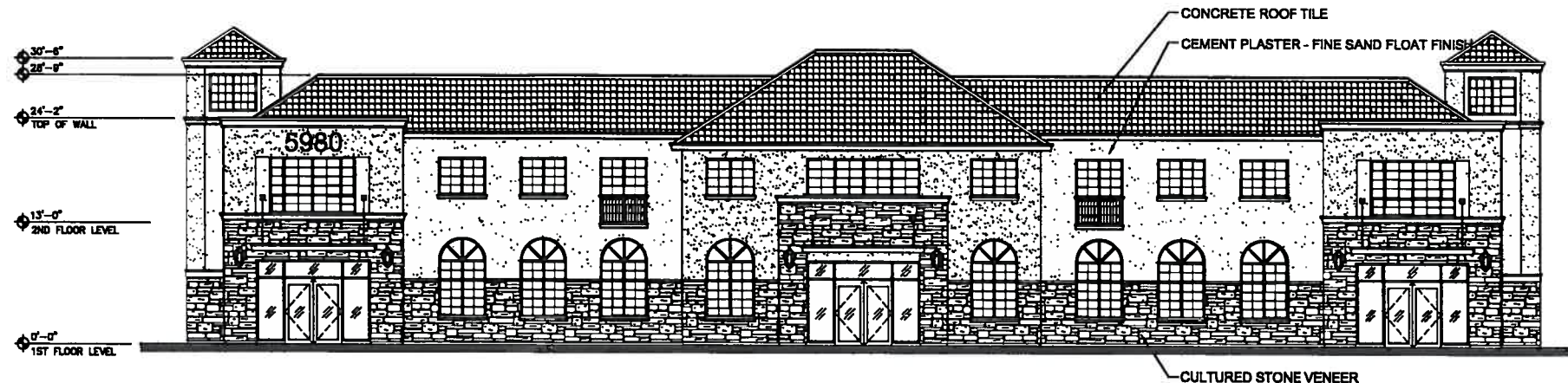
EAST ELEVATION (FACING PARKING LOT) SCALE: 1/8" = 1'-0"
