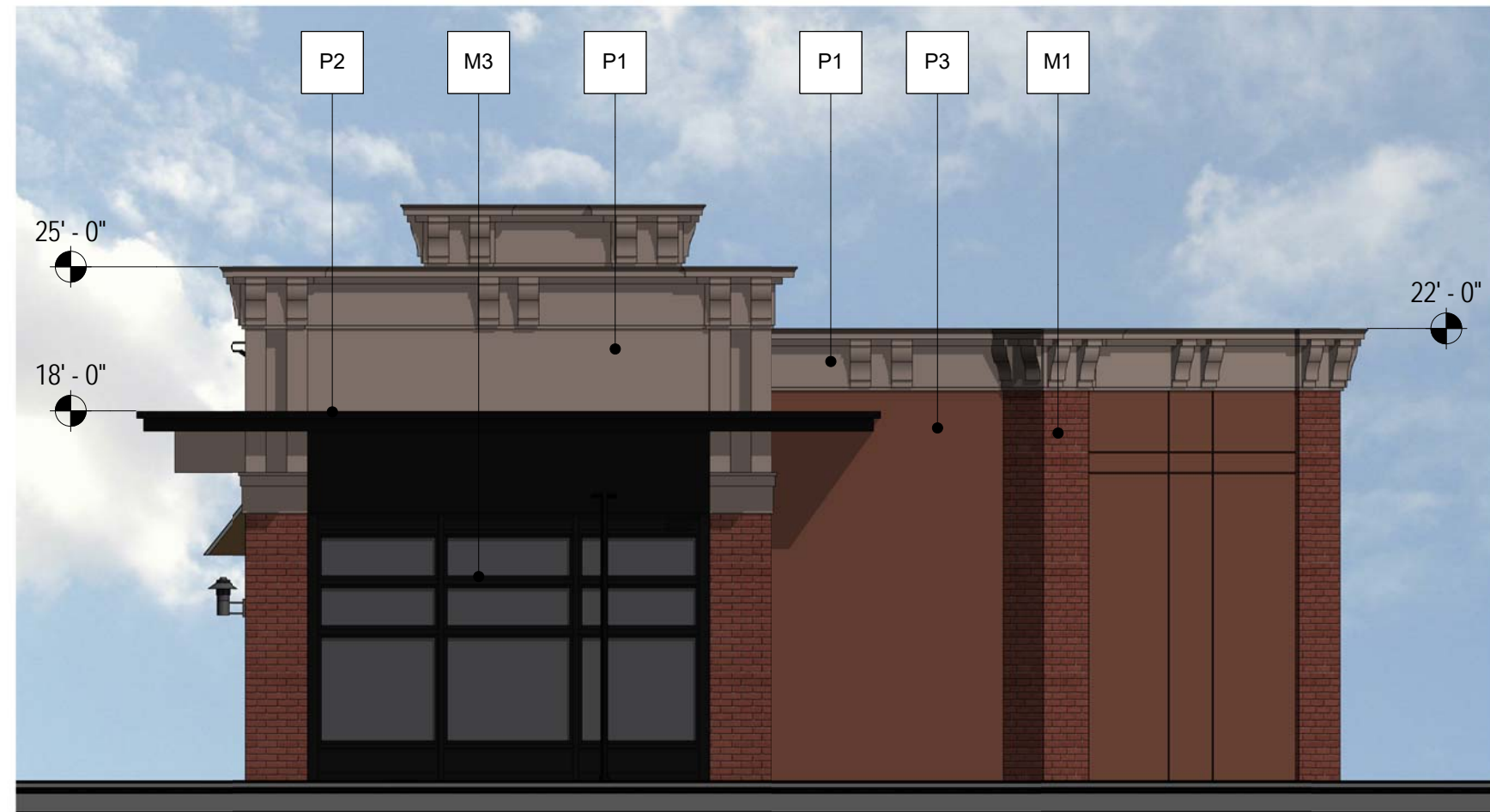
1 BUILDING A EAST ELEVATION 1/8" = 1'-0"
