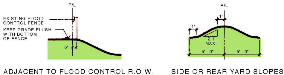
Figure 3-16: Side and Rear Yard Landscape Adjacent to Flood Control Channels
