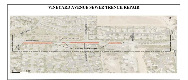
**PROJECT DESCRIPTION**: This project will repair the sink holes along the 10-inch sanitary sewer alignment on Vineyard Avenue, between Sauterne Way and Vista Diablo Court, by the compaction grouting method.
