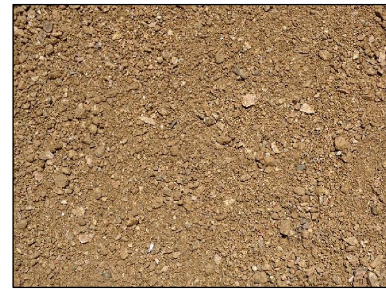
DECOMPOSED GRANITE SURFACE
