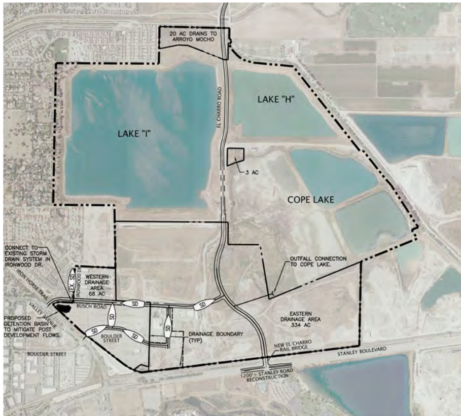
Figure 8.4 - Storm Water Drainage Plan
